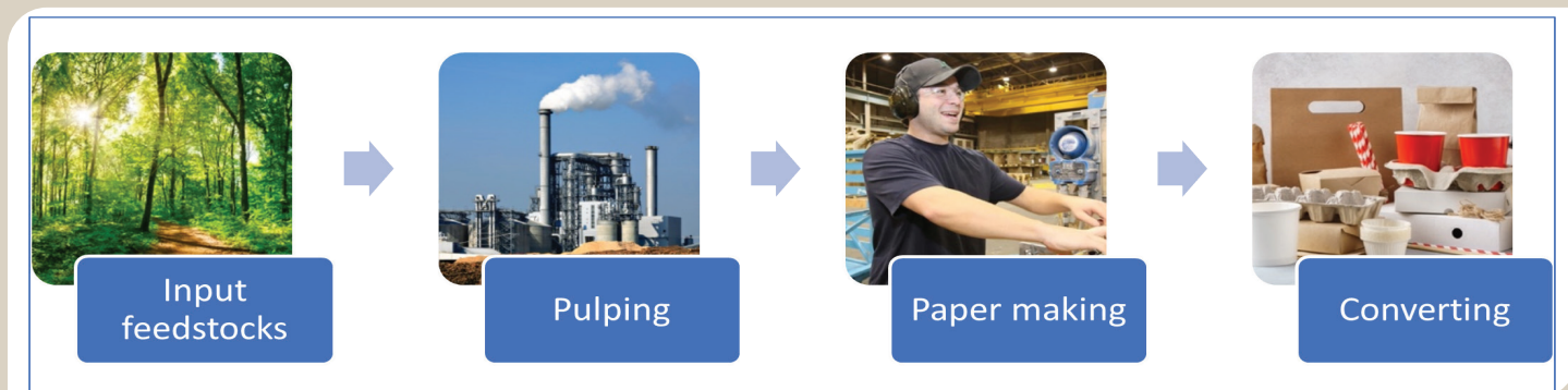
Figure 1. The process flow for manufacturing converted products (input feedstocks in the paper industry are increasingly recovered paper products such as old corrugated containers and mixed paper)
